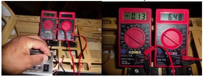
Second Servo Not Good!! 6.03 volts and .53 amp draw jumped to 1.5 amps After Cleaning and lubricating the gear train on both Servos 6.58v - .01 amps At rest
