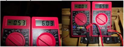
6.44 volts and .13 - .80 amps while being activated, this is normal especially when the voltage drop wasn't drastic while activating them.
