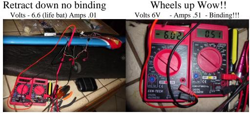
Notice the big drop in voltage the battery is heavily loaded.
