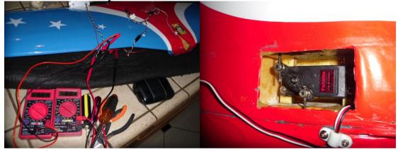
I used a servo tester instead of the receiver and battery in the plane. For each application there are shortcuts that can make the troubleshooting and repair easier.
