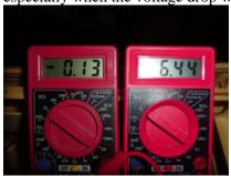
This testing can be adapted to test motors or any other electrical part in the system. Plugs and wiring can be tailored to fit. The limit for most cheaper meters is 10 amps.
