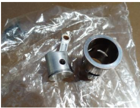
O.S. Hyper 50 Heli Motor parts after cleaning. Had 50 hours runtime.
