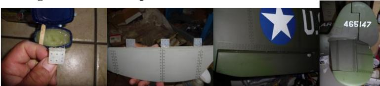
4) After the glue is completely dry on the control surface apply more Vaseline to the center of the hinge on both sides then glue the control surface with hinges into the stationary side. Press the two halves tightly together. The excess glue will come out of the center. Clean it up with Rubbing alcohol and a rag as it comes out. Work the hinge a little as it's drying to help circulate the Vaseline.
