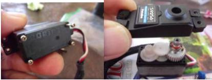
To keep gear train in tact while you take the top of the case off you have to push the top gear/shaft down (that holds the servo arm) before removing the top case. Your trying to push the bearing down along with the main gear to release the shaft. This way the gear train stays together when you remove the top case. Sometimes the bearing stays in the case.
