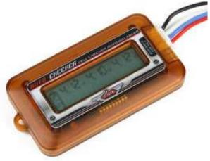
I consider cell balance to be acceptable if all cells are within .04 volts of one another on a three cell battery or .05 volts on four or more cells. As a practical matter you probably will not be able to get them closer than .02 volts.
