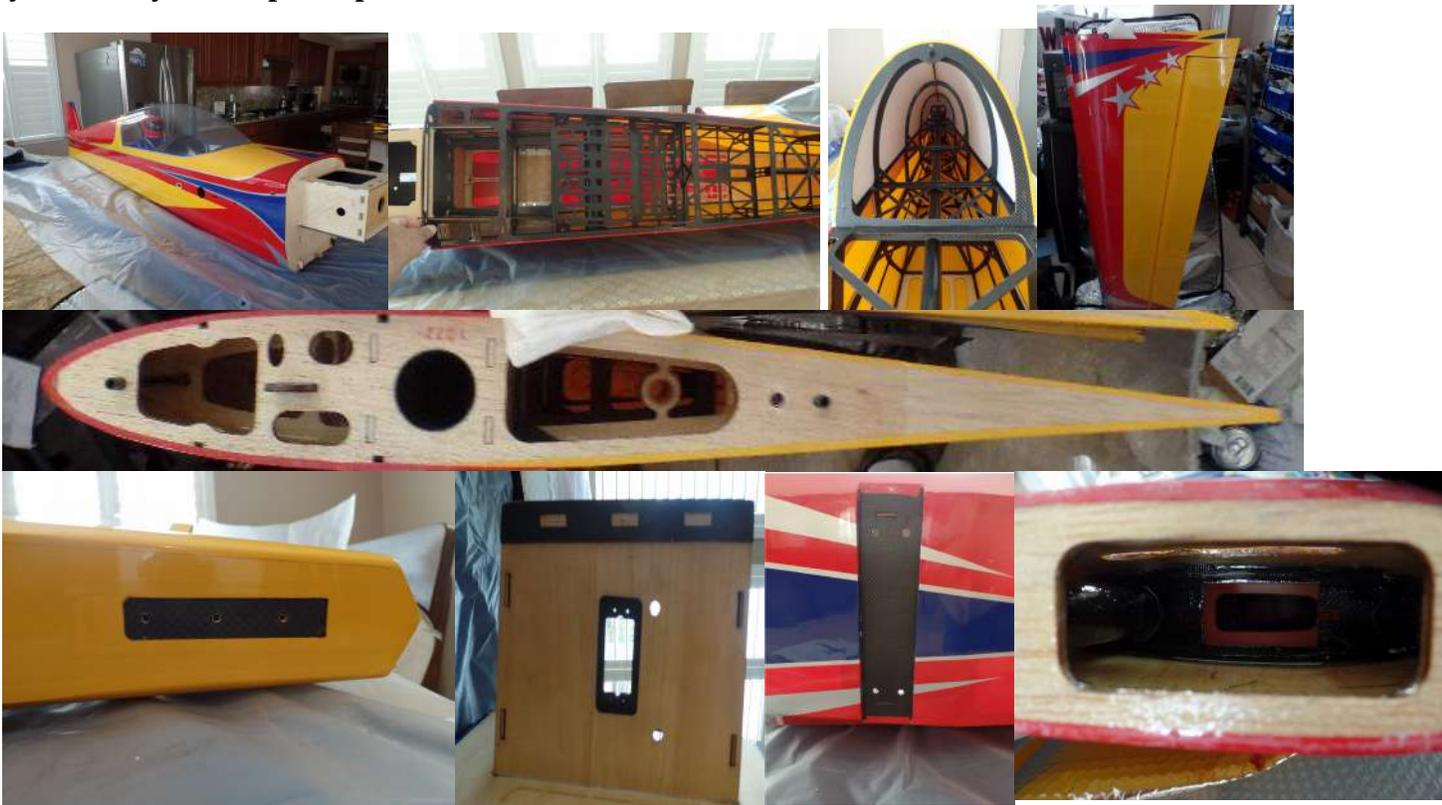
**A really nice feature that speeds up assembly is that the hinges are pre-installed and glued in- on all the control surfaces. The quality of the hinge installation is excellent and better than I can do. Yay!! I hate doing hinges. Control Horns, ball links and control rods come with the plane.**
