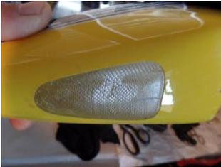
**After the Epoxy has dried remove the masking tape and plastic. Remove glue that had flowed through the masking tape and stuck on the outside of the canopy. The Epoxy is still pliable after one day and can be removed by rolling it off the painted side of the canopy. Some less flexible types of Epoxy are impossible to get off.**
