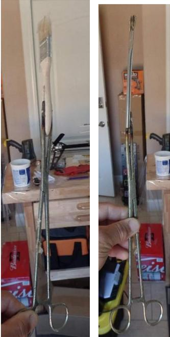
By Clipping different size brushes on to a Hemostat you can get into hard to reach places Like into a Fuselage or inside a wing.
