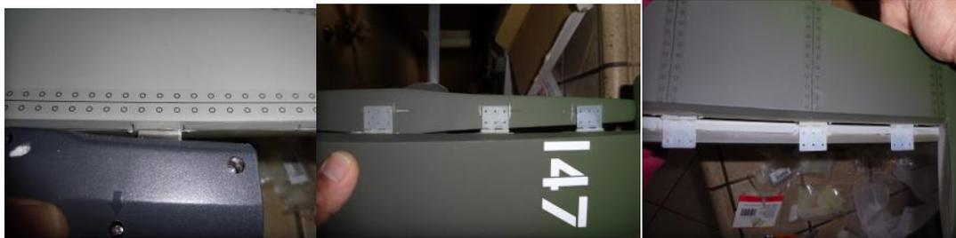
If there is no CA hinge opening at all simply run a pencil down the center of the surfaces before marking the positions of the hinges and cut the slot from scratch.
