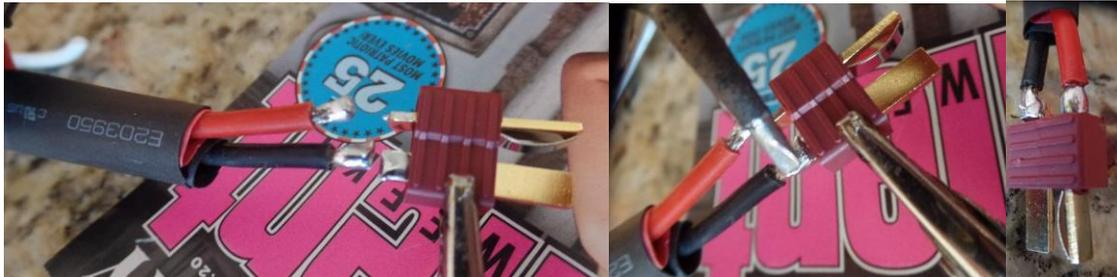
Apply heat to the connector lug for a few seconds then drop the wire on. Add enough solder and heat to make a good solid connection. The Helping hand's alligator clip can be used to clip the wire on the lug while feeding in solder. This makes the job much easier especially for thicker wire. You can go back and heat it up after taking off the clip - real quick, to get a nice solid silver ball.
