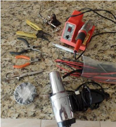
Basic Soldering Tools and insulators
