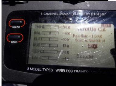
**Throttle Cut Menu options** - Assign the Switch you want to use and the set amount of throttle you need, by adjusting the percent amount, when the switch is activated. A low setting to cut the engine on a electric model and a little bit higher setting for a engine powered plane for a robust Idle. Check your radio's end point adjustments and linkage throws on the plane if there's a problem getting this to work.
