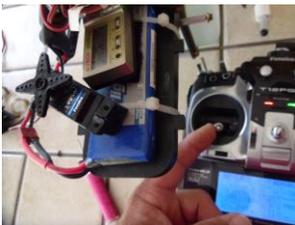
The Servo should be smooth along the travel and not bind. Grab the servo arm and activate the servo making sure it can work slightly loaded down without stripping.
