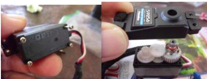
To keep gear train in tact while you take the top of the case off you have to push the top gear/shaft down (that holds the servo arm) before removing the top case. You're trying to push the bearing down along with the main gear to release the shaft. This way the gear train stays together when you remove the top case. Sometimes the bearing stays in the case.
