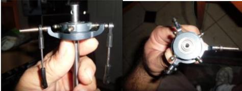
There are some different layouts. This is a CCPM setup for a Trex 500 electric.
