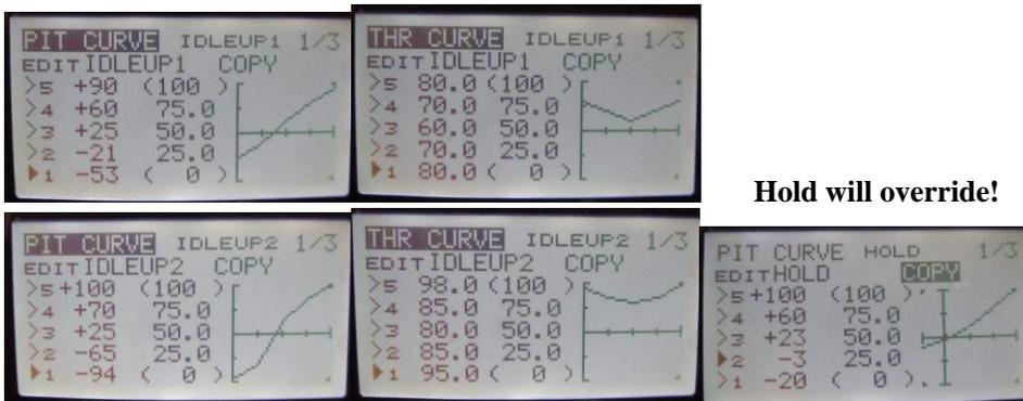
Moving the Idle up switch on the radio up one click will take you to the Idle-up 1 mixing mode. Two clicks and you'll be in Idle-up 2. In these modes the negative pitch at low throttle will be increased giving you more negative pitch on the rotor blades for flying inverted for doing stunts. -5 degrees is good for loops and rowels and slow inverted flying. -10 on Idle-up 2 for high speed 3D stunts.
