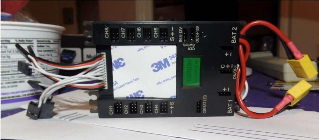
The Black unit has 8 Channel outputs with the ability to power two servos on each channel, however the servos have to be matched to operate off the same channel. Otherwise a device such a Matchbox which is a multiple servo synchronizer has to be used for 2-4 servos working on the same control surface of a Aileron, Elevator or Rudder.
