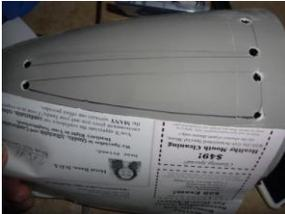
4) Cut out your Cowl ventilation holes using a circular bit on the Dremal tool.
