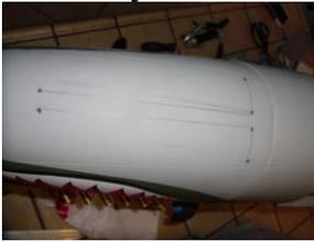
2) Cut holes out with a Dremal tool using a round Dremel bit. Don't use a drill bit.
