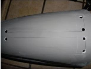
3) Remark the lines for cutting out the opening. This time mark the cut lines from the outside of the holes. Junk Mail or a regular ruler work good for drawing the line.
