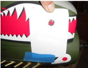
5) Cut out the hole out with a Dermal tool where you marked the opening.
