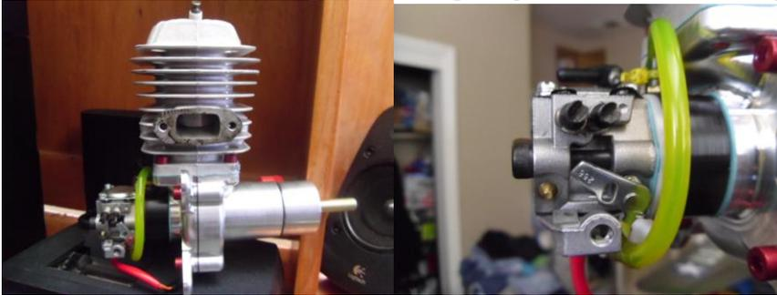
**On Most Walbro carburetors the High speed needle is located the furthest from the engine cylinder or closest to the choke. The Low speed needle is next to it and is closest to the engine cylinder.**
