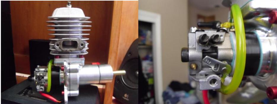
**On Most Walbro type carburetors the High speed needle is located the furthest from the engine cylinder - closest to the choke and the Low speed needle is next to it and is closest to the engine cylinder.**
