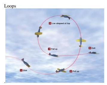
At cruise, push the nose down, gain speed and then gently pull up.
