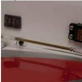
To make custom size pushrods I purchased some 2-56 threaded pushrod from the local hobby shop and cut it to the size needed, which was only about 3 to 4 inches long. They come in 12" lengths so you can make up any size you want. The threads run all the way up and down the rod.
