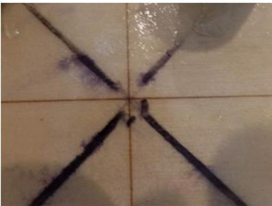
Using the markings as a reference get your engine into position so the center of your engine aligns with the center mark and the 45 deg lines, If your engine mount is perfectly square to the center this is very easy. In my case the mounting legs on the DLE 61cc engine are in a off pattern - like most gasser engines. do a visual estimation. and mark ----
