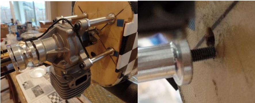
**Align the engine to where you think it should mount while tightening the one bolt.**
