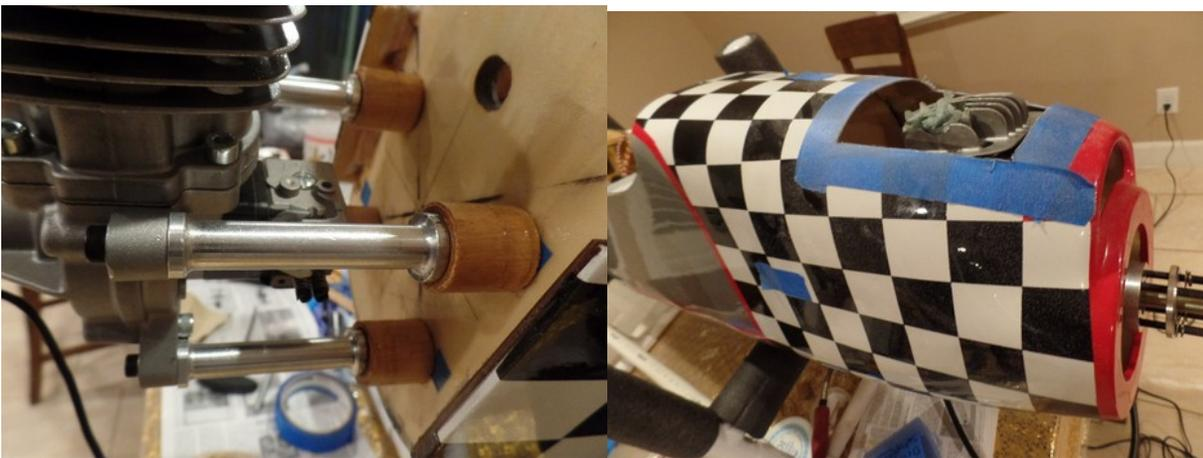
Engine fully mounted with Spacers
