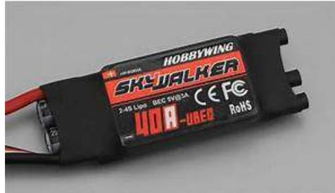
**A little more Amp handling capacity is better** – If the plane /motor calls for a 20 amp ESC it wouldn’t hurt to get a 30amp. The extra amp handling capability will come in handy if your pushing the airplane. The weight difference is small. Manufacturers will just put in whats required to reduce cost in a RTF plane.
