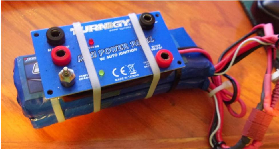
This is a lightweight easily portable unit that will supply 12 volts to the Starter or Fuel pump and 1.5 volts to the Glow Plug and also has a Glow Stick charger. To build you strap one or two battery packs that supply a total 12-15volts with Zip ties on to a mini power panel unit. I used a Hobby King Mini power panel - \$7 plus shipping:
