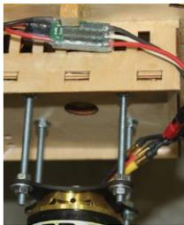
This is a big motor requiring a large speed control and unfortunately, this one isn't up to the task. Adding to the problems is the small gauge wire and adapter using un-insulated bullets.
