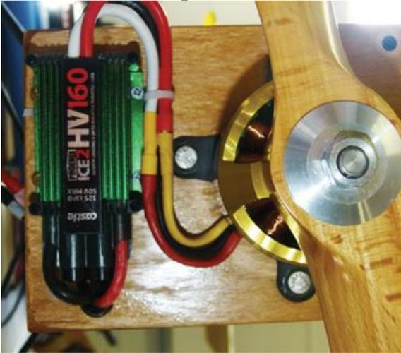
Note the securely attached speed control for this big power system and how the connections are well insulated and secured. Short wire runs and a protective grommet in the firewall, where the wires pass through, ensures no shorts over time.
