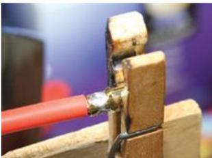
A good soldered joint between the wire and 6mm bullet will handle a lot of current. Note that there is no excess solder running all over the outside of the bullet and the joint is shiny clean.
