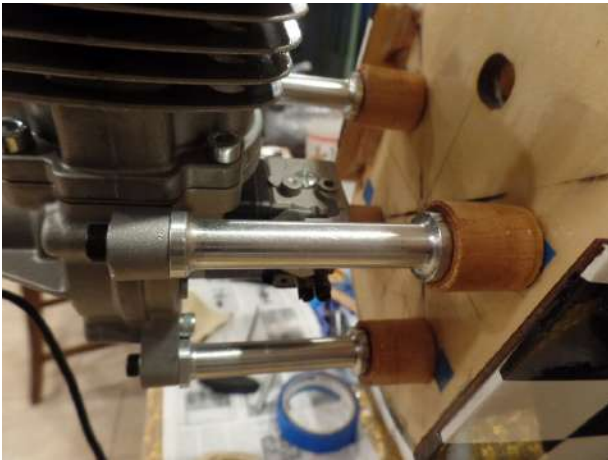
Engine fully mounted with Spacers
