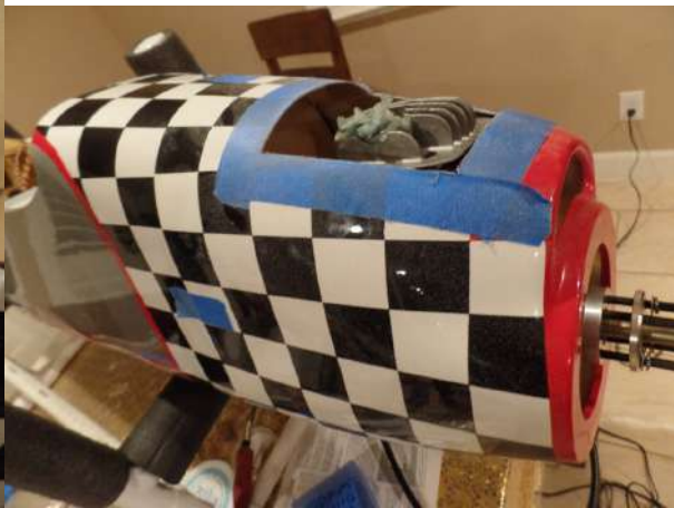
Cowl cut for cylinder head and muffler
