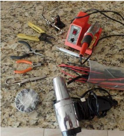
Basic Soldering Tools and insulators
