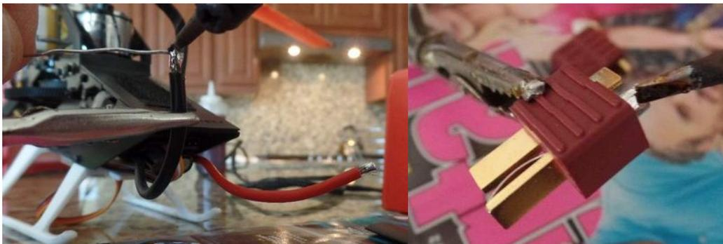
Tinning the wire tips for the connector      Tinning the connector lugs
