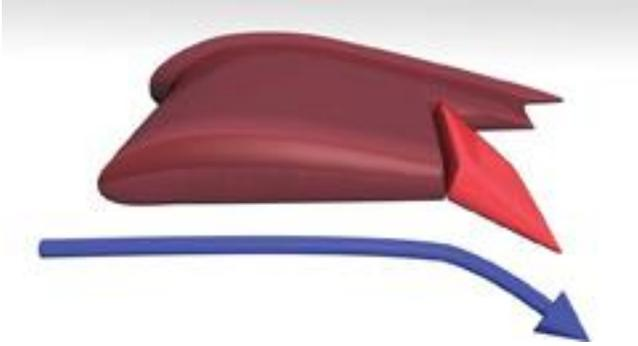
**Plain flaps lower the wing's trailing edge increasing its curvature and, therefore, its lift.**
