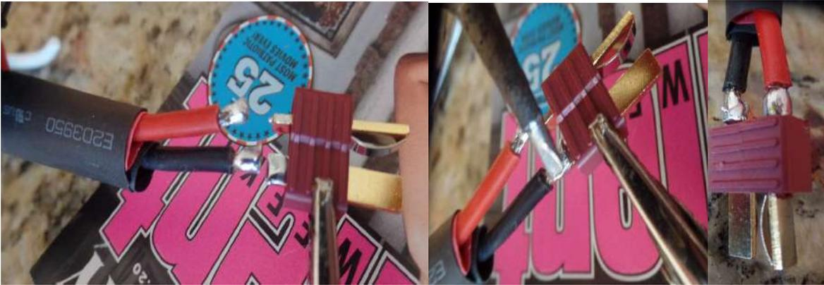
Apply heat to the connector lug for a few seconds then drop the wire on. Add enough solder and heat to make a good solid connection.
