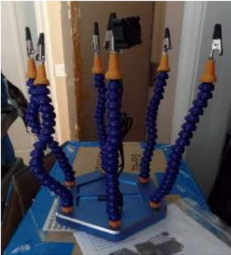
This Helping hand Setup even has a USB powered Fan to cool off your connection joints after soldering. Say goodbye to burning your fingers!
