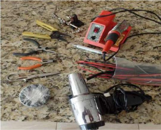
**Basic Soldering Tools and insulators**
