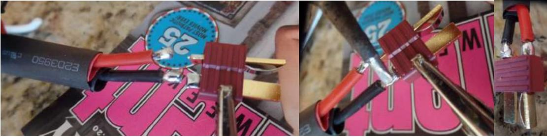
Apply heat to the connector lug for a few seconds then drop the wire on. Add enough solder and heat to make a good solid connection.
