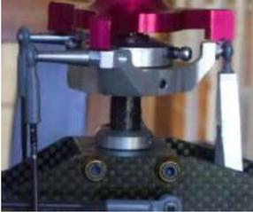
140 Degree CCPM with a Leveler tool on the shaft
